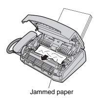
When the recording paper has jammed near the recording paper exit:
